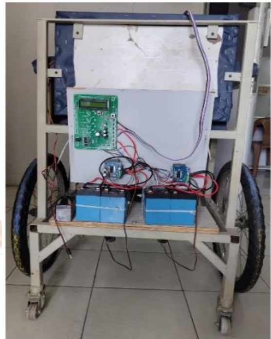
Figure 4 Control Unit of the Wheel Chair
