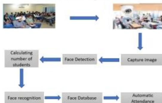
Figure 2:Block Diagram of Attendance System
