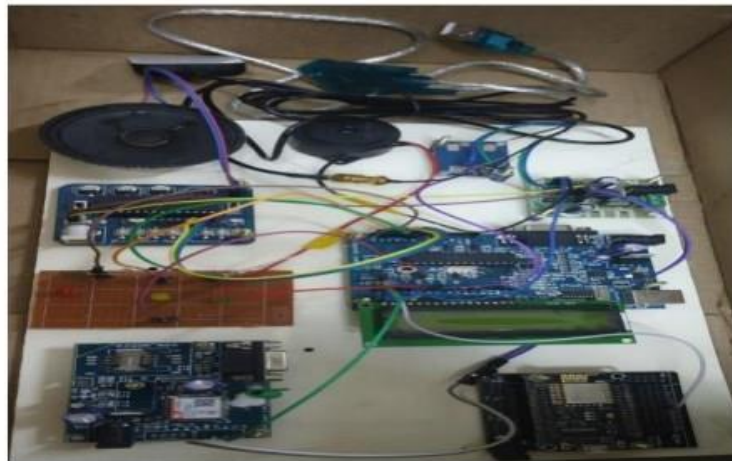
Figure 12: Hardware implementation of RSSI
