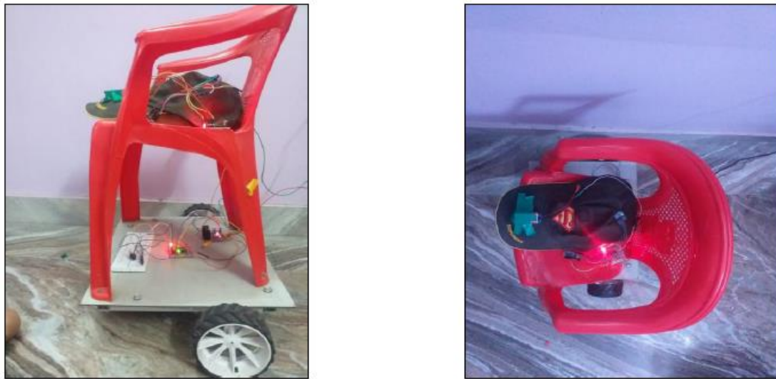
FIG 11: Head Gesture Controlled Wheelchair Based on RFID
