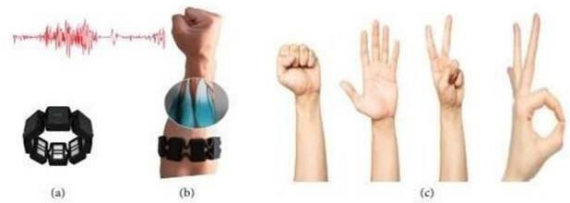
FIGURE 1: Myo armband: (a) Myo and EMG signal, (b) muscle activities on the forearm, and (c) gesture.
