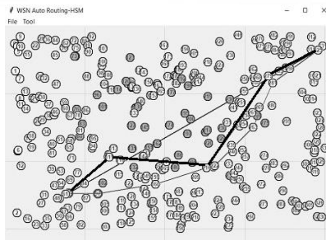
Figure 5 shows the data path in dark, thick lines and the acknowledgement path outside the data path in thin lines. The grey-shaded nodes indicate a low battery state and are unable to retransmit and allow the higher-delay nodes to participate in routing.
