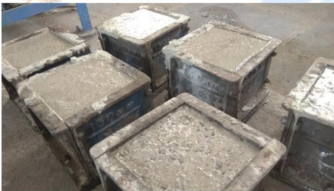
Fig -1 : Casting of Concrete blocks
