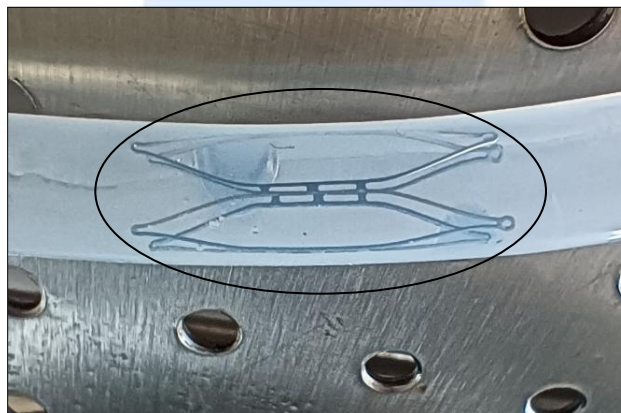
Figure.06 The implant returning to its original shape after the deployment procedure.
