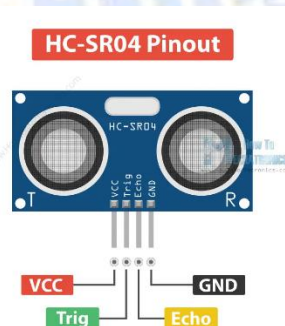
Figure 1: HC-SR04 Ultrasonic Sensor Pinout
