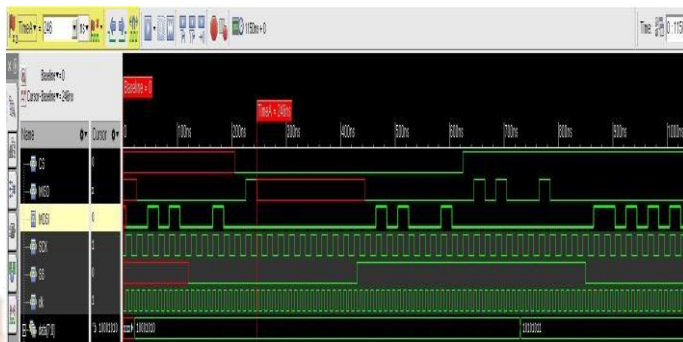
Figure.11 Simulation waveform of SPI
