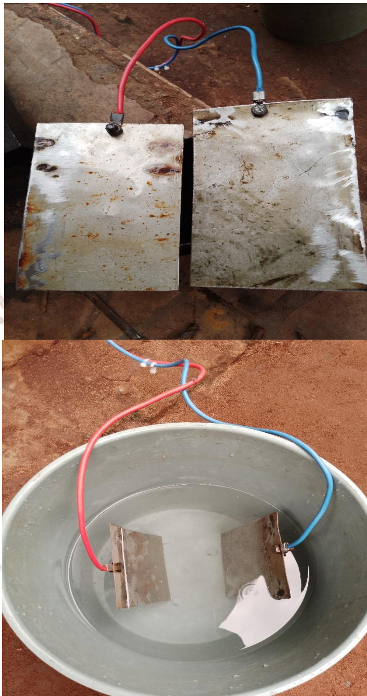
Figure 2. Diagram showing two sheet metals used as prototypes of the cathode and anode in the experimental set up
