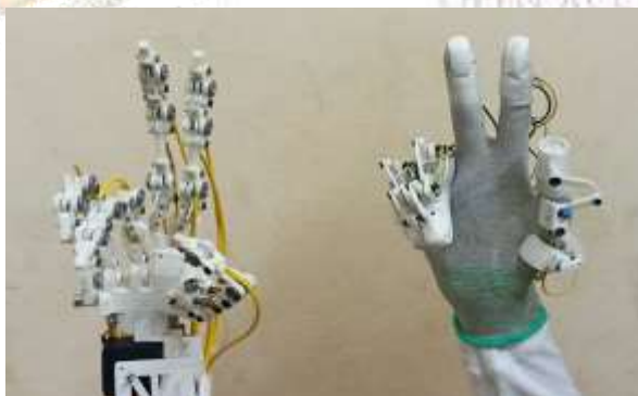
Fig 6.1 Result of the robotic hand imitation of the peace hand sign.
