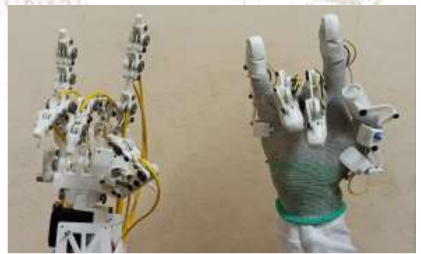
Fig 6.2 Result of the robotic hand imitation of the rock and roll hand sign.
