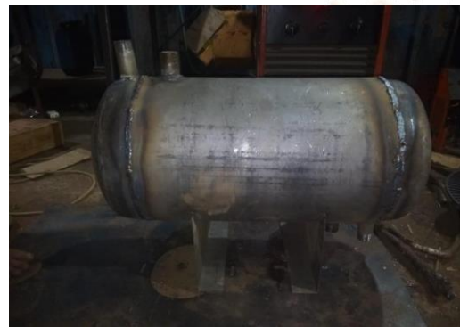
Fig.4 Manufactured Prototype of heat exchanger
