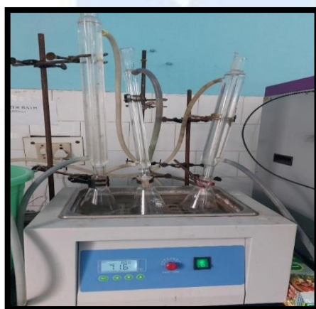
Fig 5: Heating of conical flask under condenser
