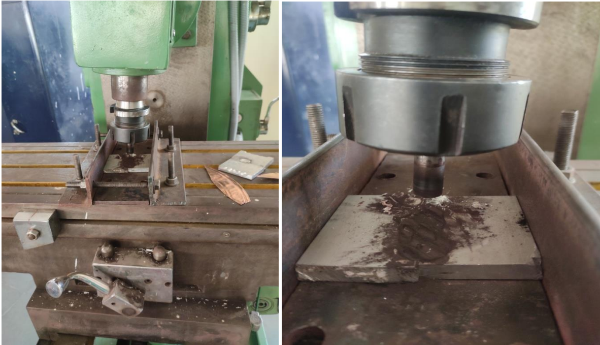
Figure: FSW on Milling Machine
