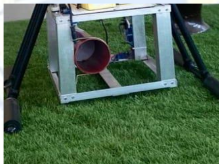
Figure 4 Assembly of Dropping Mechanism
