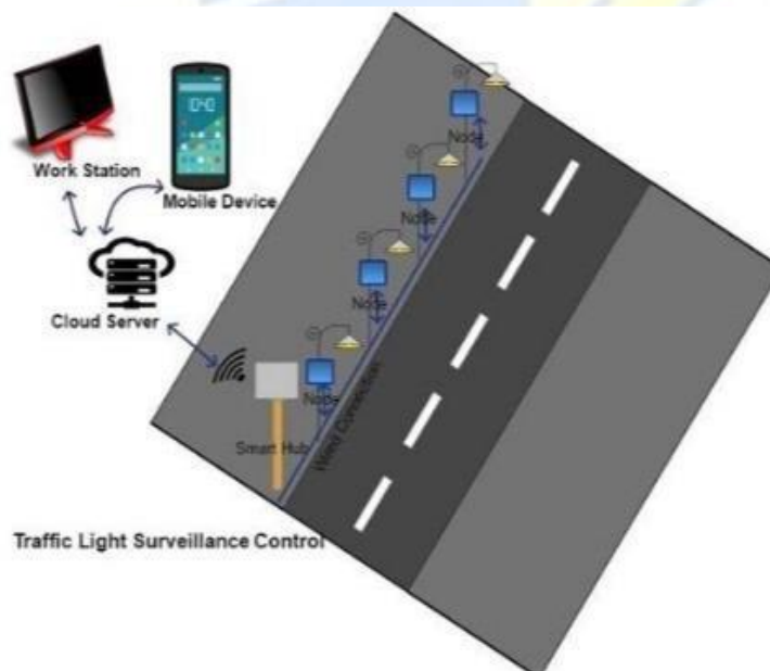
Fig. 5. Block diagram of Wi-Fi based surveillance and control system (One directional)
