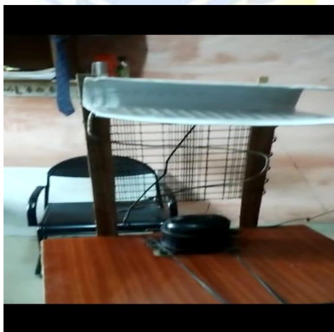
Fig.1 Vapour compression refrigeration system
