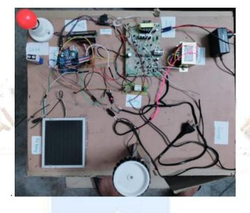
The rectified output is given to the exciting coil of the 2c relay. Normally the plate is attached to the NC pin of the relay under not excited condition. So we have attached the NO (normally open) pin to the main supply, so that in case of main power on, the supply is provided by the main to the hospital.
