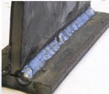
Figure 2 Transverse fillet weld joint
