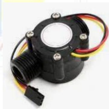
Fig 4. Water flow detector
