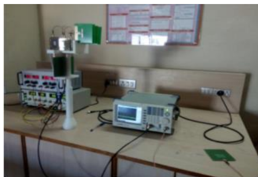
Fig. 1.3 Antenna phased array Experimental setup at 2.4 GHz.
