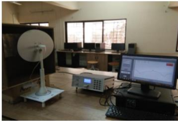
Fig. 1.5 Experimental set up for SE with stainless steel at 900, 1800 and 2100 MHz.
