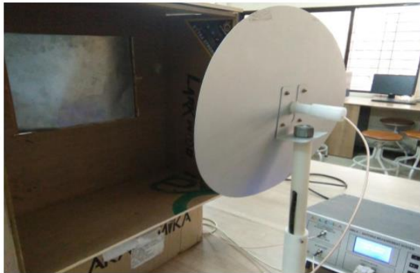
Fig. 1.6 Experimental set up for measurement of SE with aluminum shield
