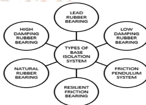
Fig. No. 2: Types of base isolation system
