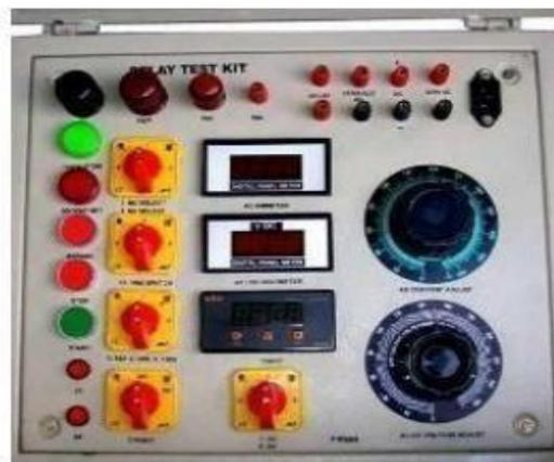
Figure-3: Secondary Injection kit
