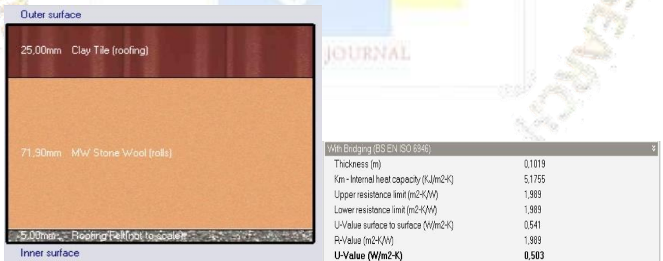
Figure 8- U value for the roof in the proposed building retrieved from Design Builder V7.1
