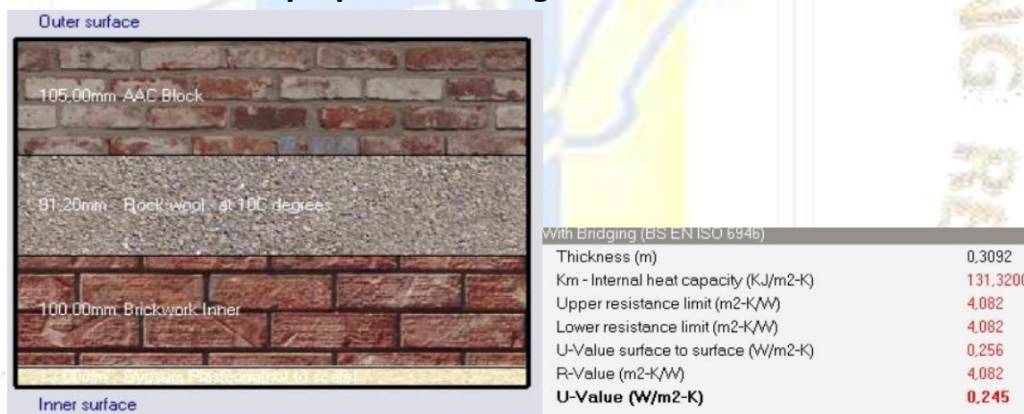
Figure 4 - U value for the Exterior walls in the proposed building retrieved from Design Builder V7.1
