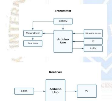
The block diagram of a Real-time person detection robot is shown above.
