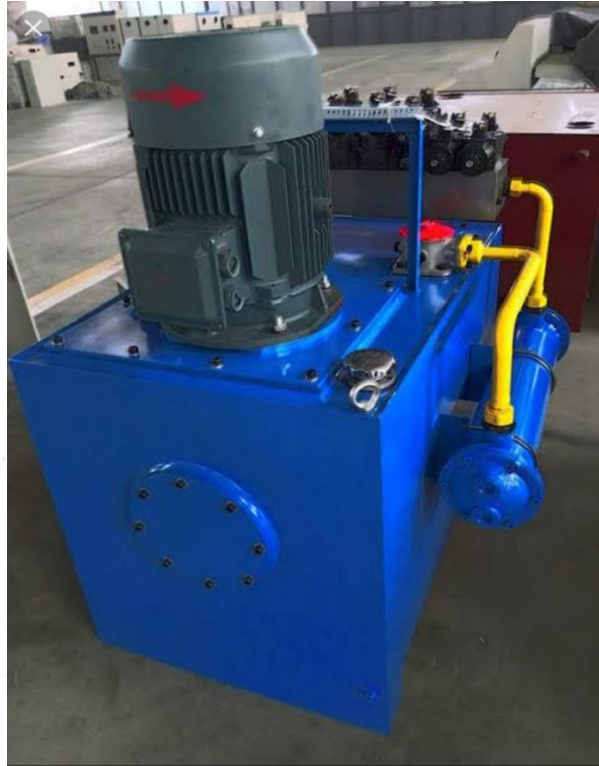
Fig 2.2.6.1 Hydraulic Fluid Tank
