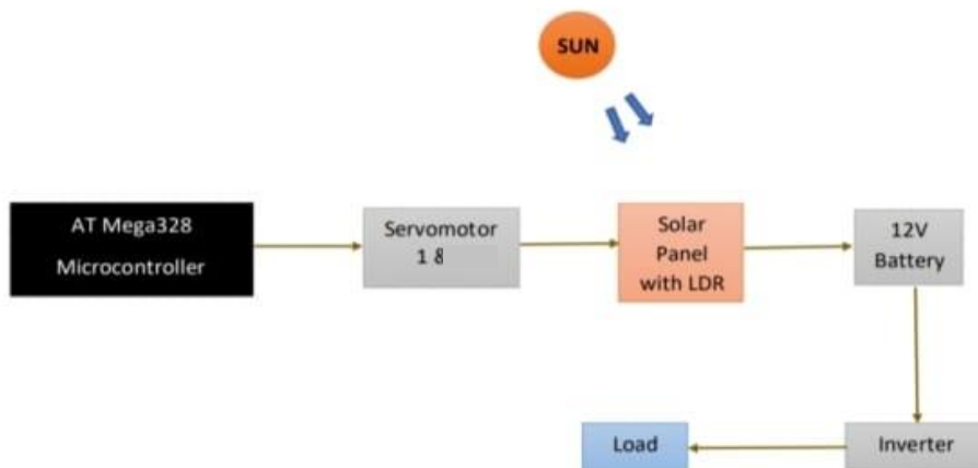
Fig.1: block diagram of the solar based inverter using microcontroller
