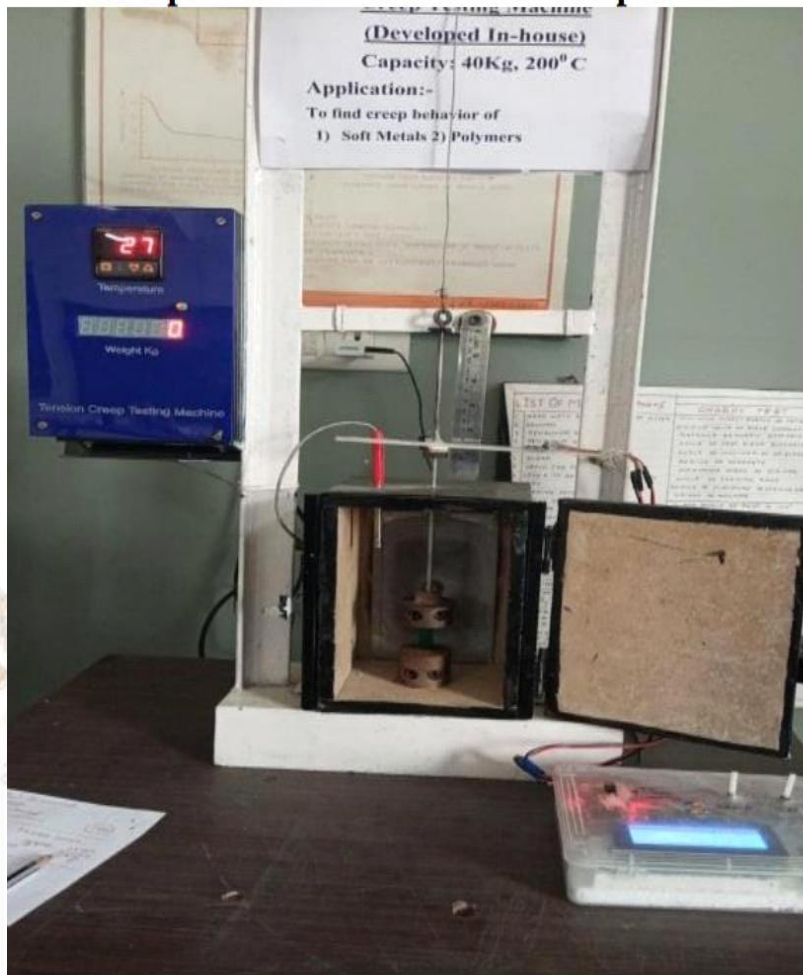
Actual Experimental Setup of Creep Testing Machine
