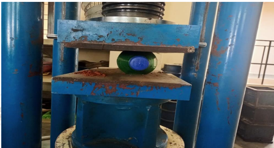
Figure 9: Load bearing test (bottle bricks)
