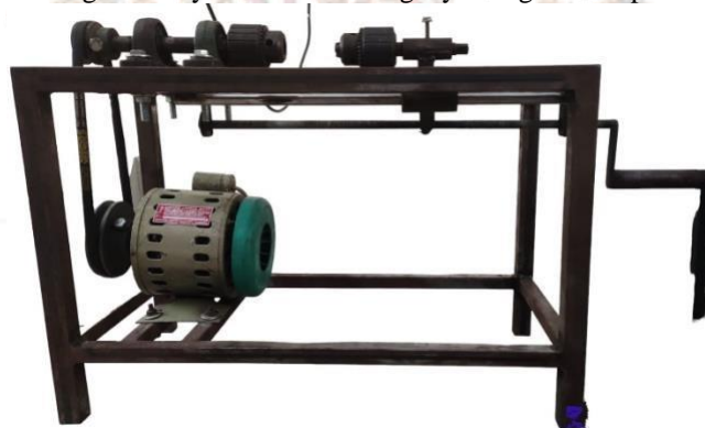
Fig.3 Rotary Friction Welding By Using Steel Pipes
