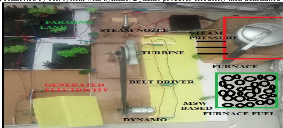
Fig 4: A prototype structure for generation of electricity by MSW Based Fuel
