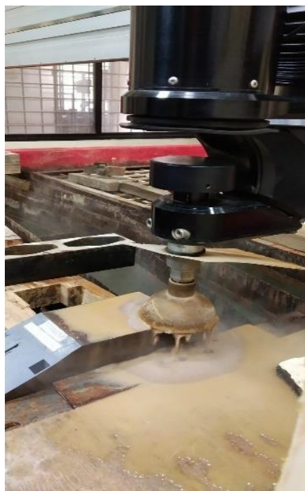
Figure 1 Setup of Abrasive Water Jet Drilling of Ti6Al4V
