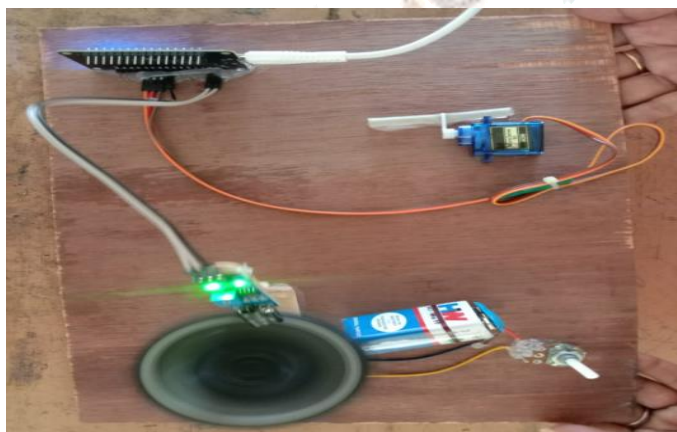
Fig 1: Servo motor stops the fuel when speed is high
