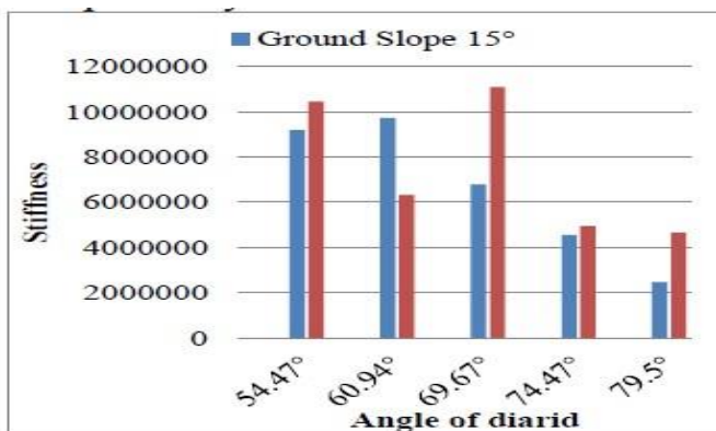
Fig 11 (n) Storey Stiffness for Diagrid building on 15° and 25° slopes respectively in X-direction
