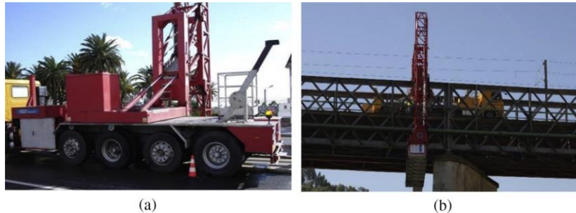
Fig. 2. Under-bridge truck: (a) parked on top of the bridge deck; and (b) platform to access below the bridge deck and the supports.
