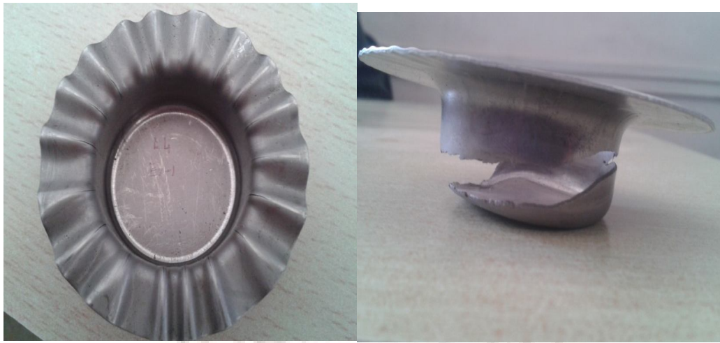
Fig.5 Before/After Machining SS 316 blank
