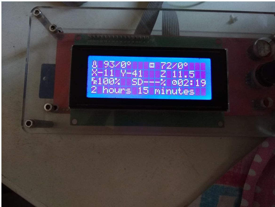
Figure 19: The module showing total time with 100% fill
