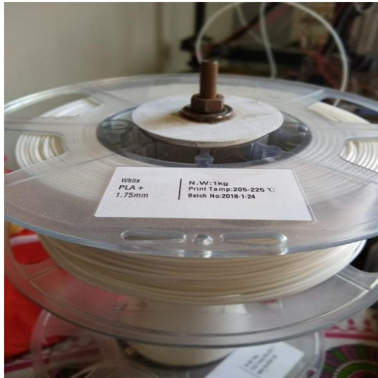
Figure 13: The PLA material reel (spool) with 1.75mm thickness
