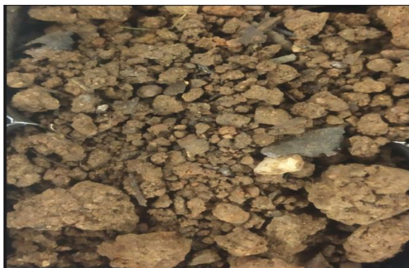
Fig. 2 Testing Soil ( Clay Soil with pH 7.00)
